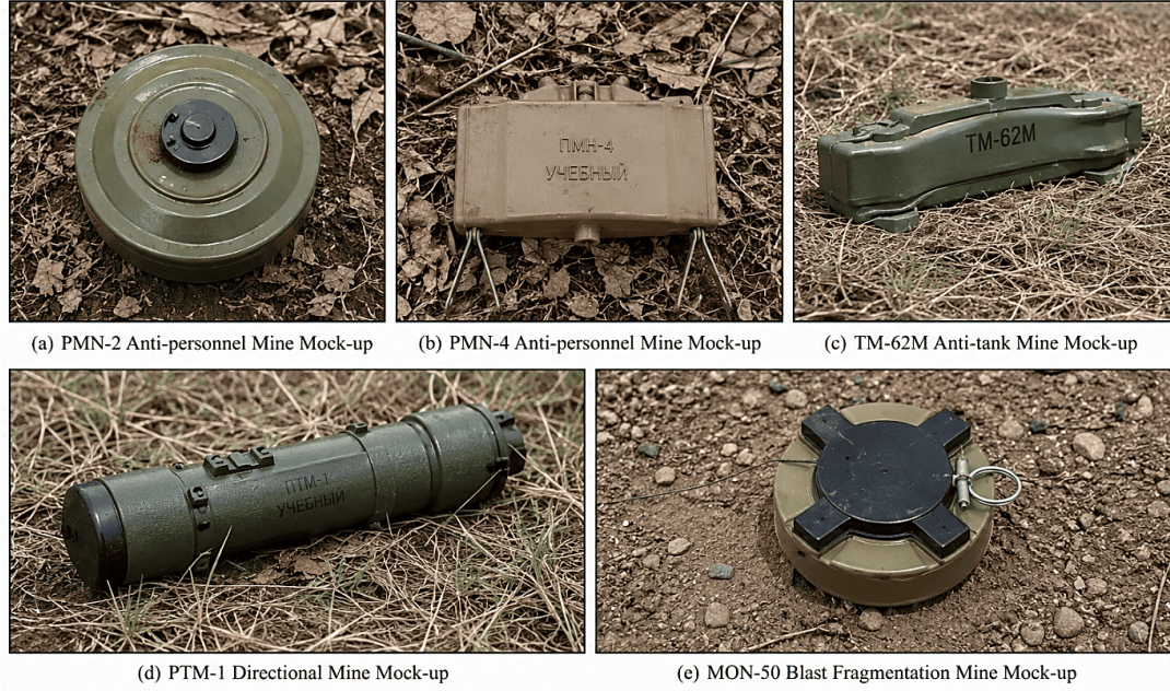
Figure 5: Examples of explosive hazard mock-ups used in experimental studies.
