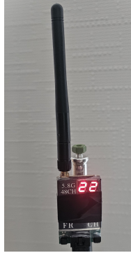
Figure 2: Reference emitter: 5.8 GHz, 48-channel analogue video transmitter configured on channel 22 ( f_{\text{VTX}} = 5752 \text{ MHz} , P_{\text{out}} = 600 \text{ mW} ).
