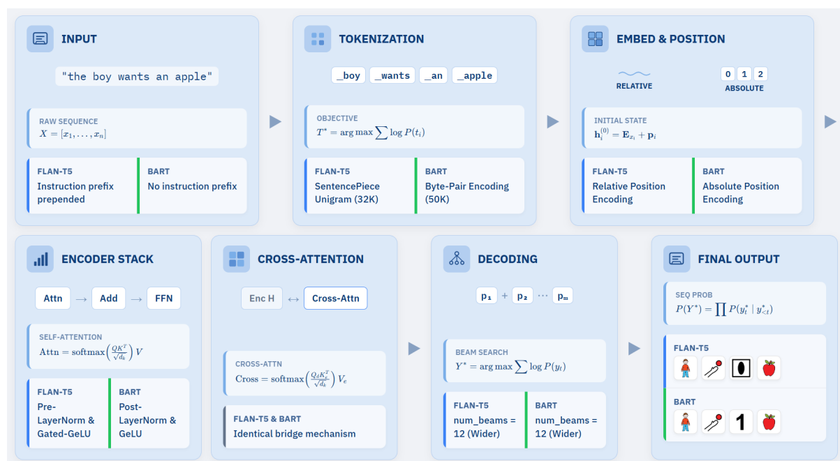
Figure 5: Comparative architecture of the FLAN-T5 and BART-based encoder-decoder transformer frameworks
