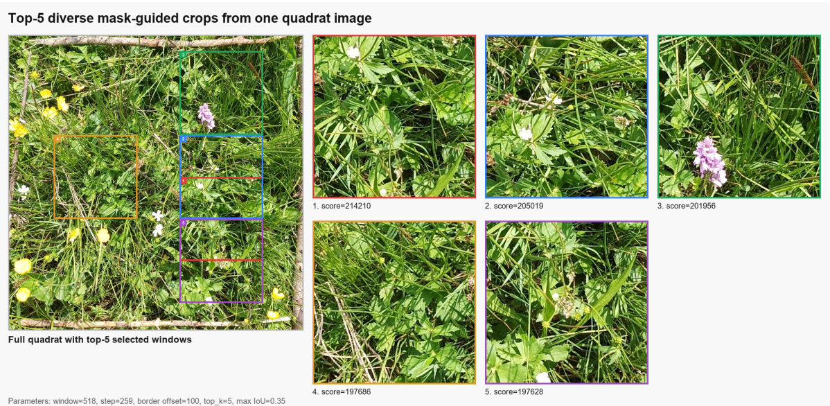
Figure 9: Example region proposals produced by the mask-guided crop strategy. The selected windows concentrate the fixed-size classifier input on vegetation-rich parts of the quadrat rather than on the full image frame.
