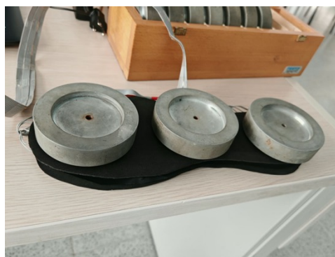
Figure 6: Initial load level of the reference masses on the heel, midfoot, and forefoot regions.
