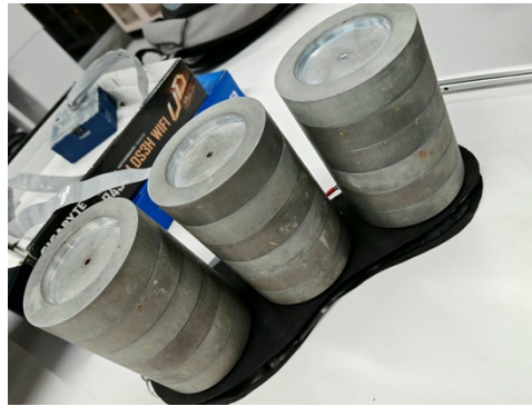
Figure 7: Maximum load level of the incremental sequence of reference masses.
