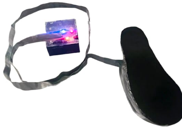
Figure 5: Integrated prototype of the instrumented insole after functional recovery.
