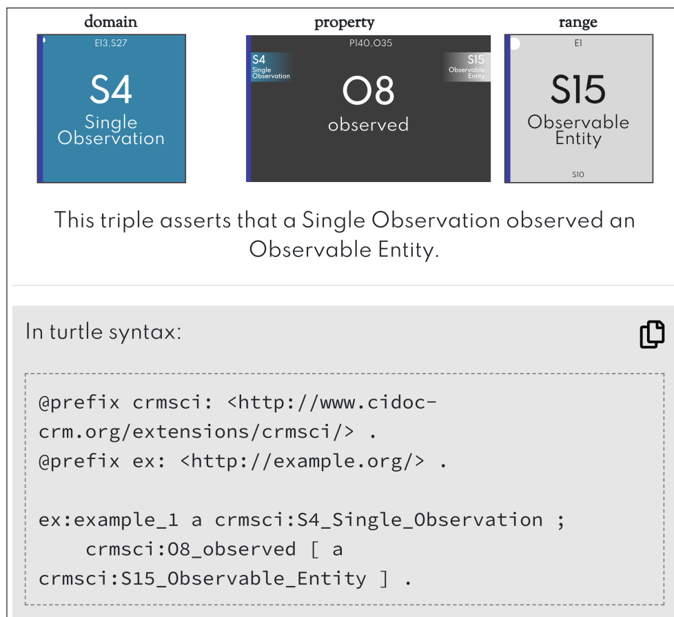
Figure 4: One-step output for S4 Single Observation, O8 observed, S15 Observable Entity: the natural-language read-back and the instance-level Turtle with the prefixes the triple actually uses. Only 6 of the 131 loaded classes are admissible in the range slot for O8 — S15 and its five subclasses — and the table dims the rest while the choice is open.
