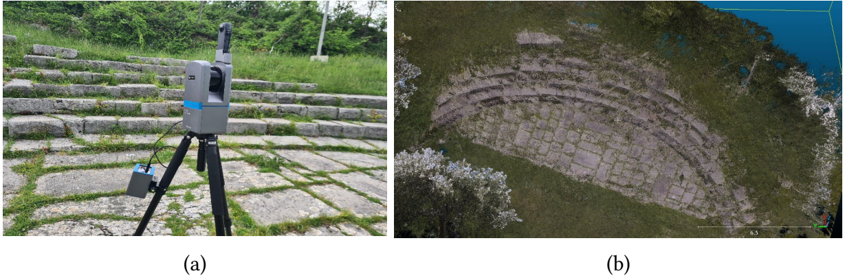
Figure 8: Acquisition by Stonex X100: picture of the device during the scans (a) and 3D points cloud (b).
