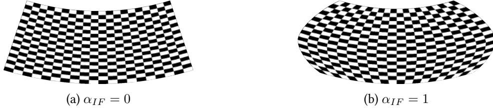
Figure 5: Shape change introduced by \alpha_{IF} \in \{0, 1\} when unrolling the model shown in Figure 1a.
