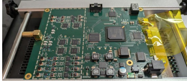
Figure 9: Installation of the USB3 FIFO chip from a donor board during the initial hexachannel prototype implementation of Waxwing in August 2025. Dimensions of the system excluding the RF connector are 131 by 103 mm while mass was less than 300 g with an RF shielding frame installed.
