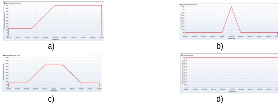
Figure 3: Load type visualization: a) Ramp; b) Spike; c) Peak; d) Fixed (source: own elaboration).
