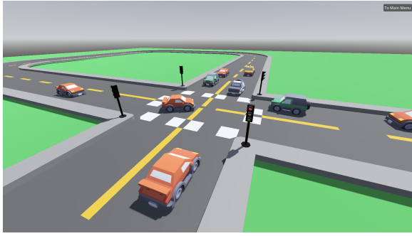
Figure 7: Left: Vehicle scenario: path-following cars combine Prolog decisions with traffic lights, local sensors and anti-deadlock guards. Right: Top-down tank scenario: agents use symbolic tactical decisions grounded by line-of-sight checks, bullets, damage and respawn.
