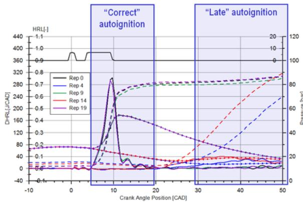
Fig. 1. Combustion patterns for individual cycles for a single test.
