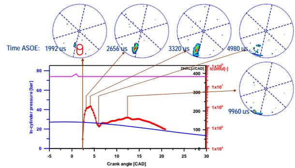
Fig. 2. Image sequence of the pilot flame combustion with cycle-resolved evolution of pressure and luminosity.
