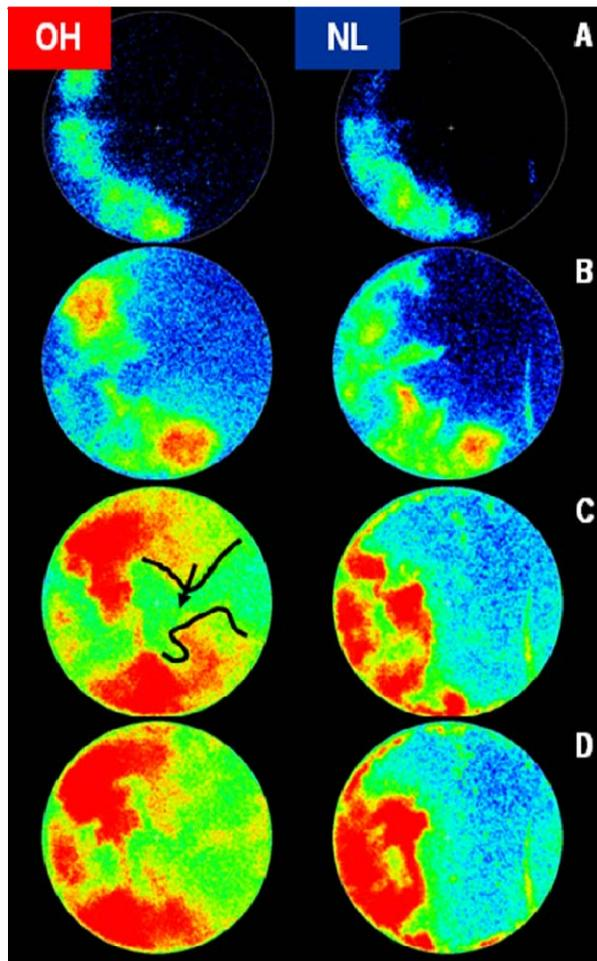
Figure 4. Simultaneous OH (left) & natural luminosity images (right) in a single cycle.
