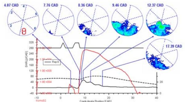
Fig. 3. - Image sequence of the pilot+main flame combustion with cycle-resolved evolution of pressure, luminosity and rate of heat release.
