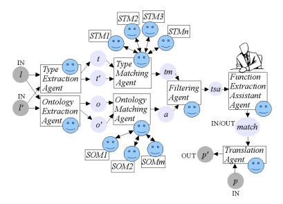
Fig. 1. The architecture of our multiagent system.
