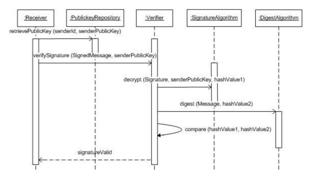
Figure 3: Sequence Diagram for verifying a signature
