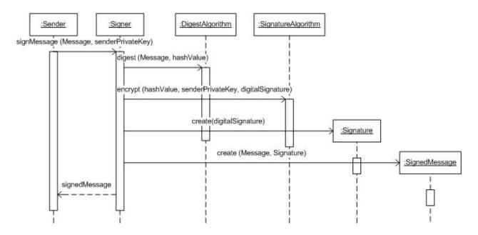
Figure 2: Sequence Diagram for signing a message
