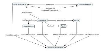
Fig. 2. Concept map with the classes and relations of the Linked Sensor Data model [1].
