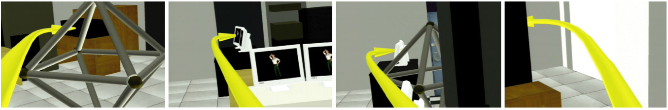
Figure 8. The Flexible Pointer Interaction Technique provides easier selection and clearer indicative pointing in collaborative environments in addition to the ability to select fully or partially obscured objects.
