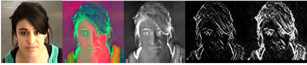
Figure 2. Different stages of the intelligibility filter (from left to right): original image, HSV image, saturation component, Sobel filter, and final image after morphological filters
