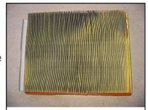
clogged air filter
