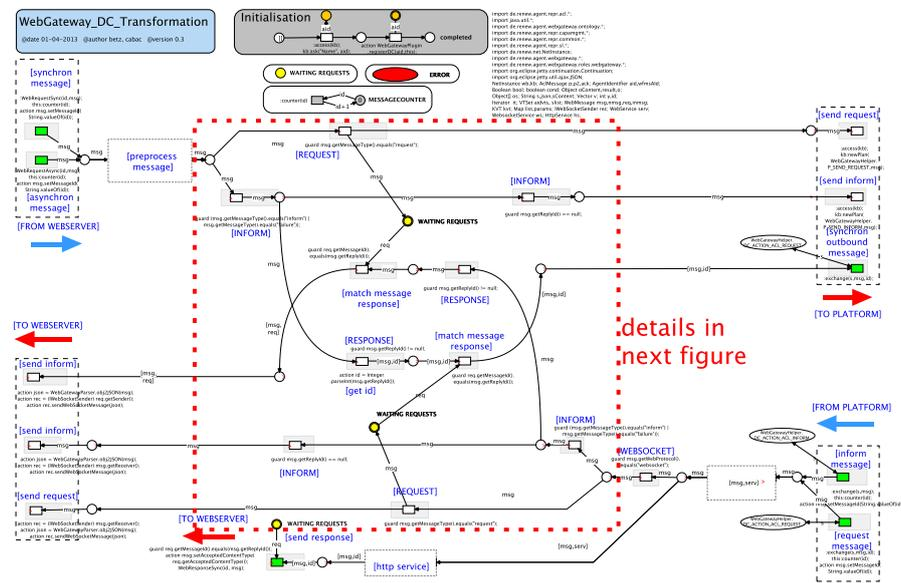
Figure 10. Implementation of the WebGateway Transformation Component.
