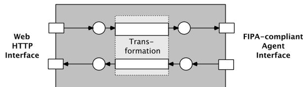
Figure 2. Simple WebGateway architecture model
