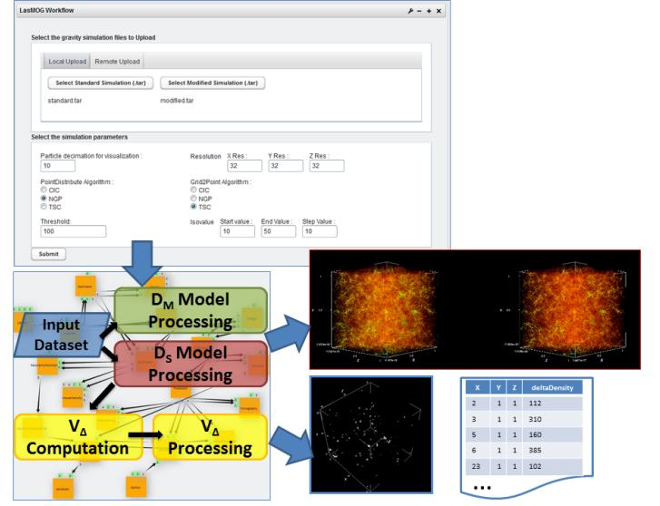
The workflow shown in Figure 8 implements a customised visualization for aiding analysis of modified GR simulations, more specifically inspecting datasets to discover anomalies by comparing appropriately with datasets coming from standard GR models. The main computational steps are summarised as follows:
